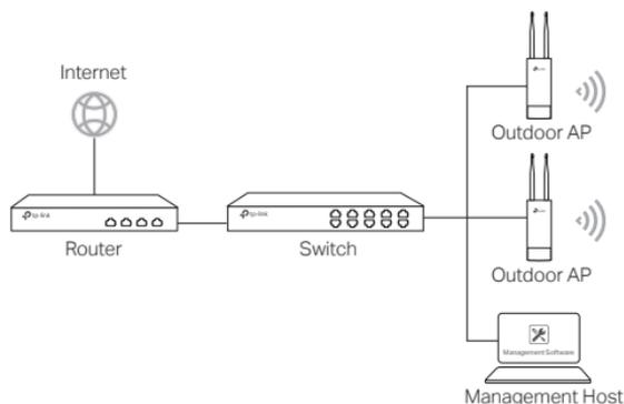
A computer running the centralized management software, which can be in the same or different subnet with the APs, is used to centrally manage the APs.
