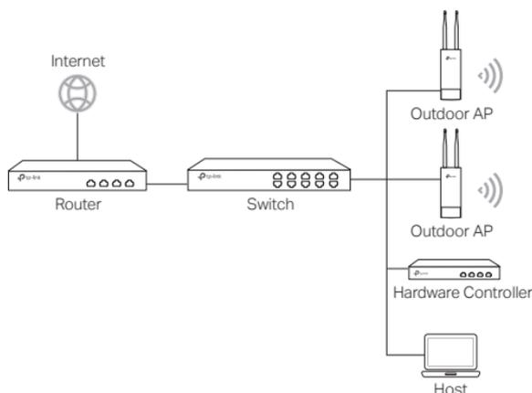
The hardware controller can be in the same or different subnet with the APs. The management host is used to log in to the hardware controller to centrally manage the APs.
