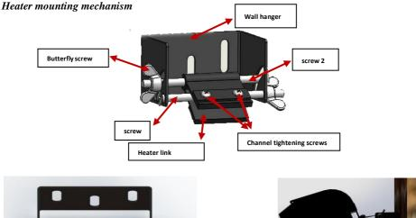
Apparatus assembly of the Infrared heater
