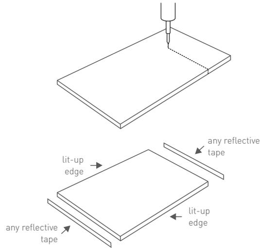
**3.** Cut the heat sink according to the size of your acrylic sheet (the full length of the heat sink is 5000mm). CNC, laser, plasma or saw cutting can be used.
