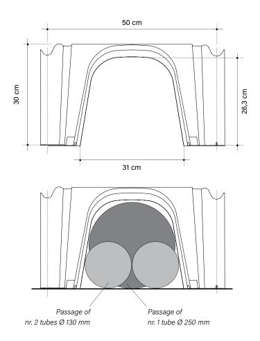
The images are only for examples. Recyclable material is allowed a size tolerance of  $\pm$  1,5%.
